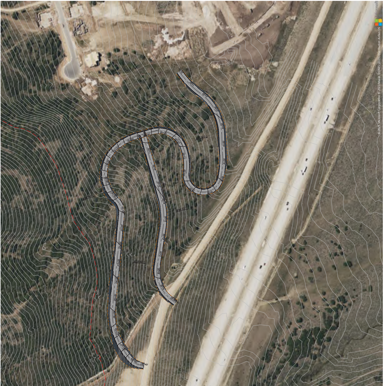
Illust. 26.1 - second option for access to the Clark Ranch West parcel. Source: Talisman Civil
