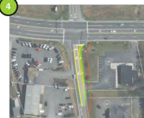
4 Dillard Rd. - new right turn lane (est. $555,000)
